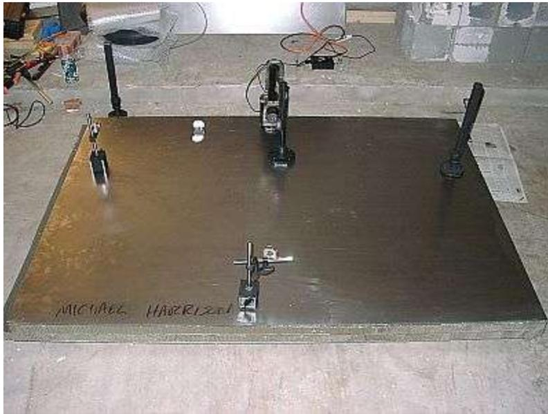
After you've done a layer or two, you should be tempted to test the top for stability. I highly recommend following this temptation. Get your laser and enough components to create an interferometer and set it up on your top. Put a few inner tubes under the top with any luck you'll find that the fringes settle quite quickly, although this depends as much on the reliability of the component mounts as it does on the rigidity of the Hexcel panel you've made.
