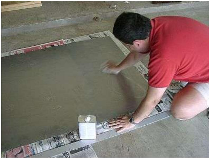
Spread out a single layer of newspaper to protect your working surface from the epoxy and sanding tools. Put a sheet of steel down and clean it thoroughly with denatured alcohol. I recommend wearing leather gloves while doing this as the alcohol is rough on the hands.
