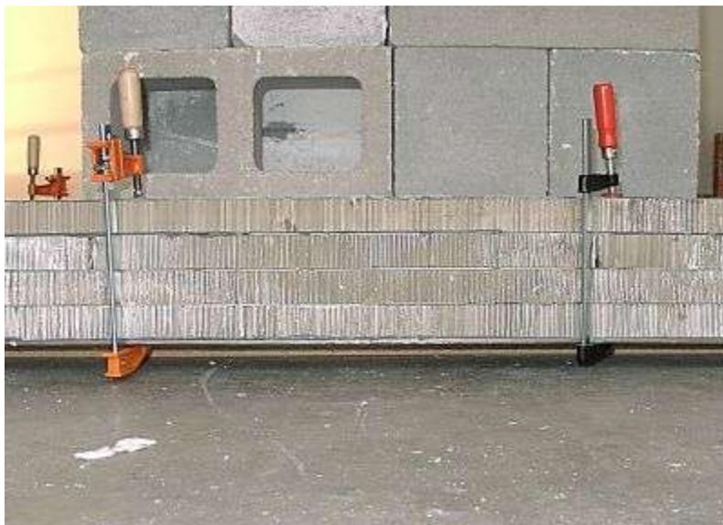
Let the layer cure overnight and then repeat the process with the successive layers of Hexcel until your table top is complete. After you've done a full panel (steel on both sides) you may want to lift the panel off the work surface slightly so that you can clamp the edges while piling weight in the middle.
